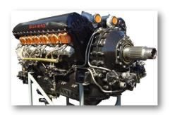
The Rolls-Royce Merlin is a liquid-cooled V-12 piston aero engine of 1,800 hp (1,300 kW).
