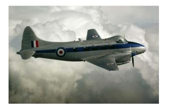
The de Havilland Dove was a twinengine, short-haul airliner manufactured between 1946-1967. It was used by the RAF for carrying VIP's, light transports and communications. It had a maximum speed of 230 mph and seated up to 11 passengers.
