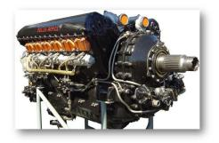
The Rolls-Royce Merlin is a liquid-cooled V-12 piston aero engine of 1,800 hp (1,300 kW). Rolls-Royce Turboprop Aeroplan Engines were named after 'Birds of Prey'
