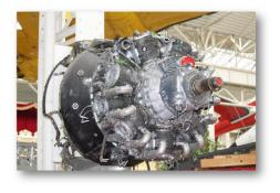
The Stirling was powered by four Bristol Hercules 14-cylinder two-row radial aircraft engines which were spaced across its midmounted wing.
